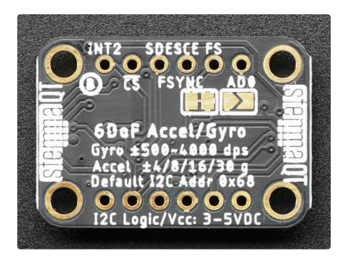
Each of our breakouts start with the sensor of interest, and in this case we begin with a hot-off-the-reel ICM20649 Wide-Range IMU. These chips are only a few mm across and have 0.4mm pitch contacts. To make it easier for folks to work with this chip, we've taken the sensor and mounted it on a breadboard-compatible breakout board.
