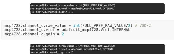
Finally for channel C, we again set the raw value to half of the maximum, so the resulting voltage should be half of the Vref voltage. We then set the Vref source to the internal 2.048V Vref, however this time we set the internal Vref's gain to 2X, making the final Vref voltage 4.096V. With the value for the channel set to half of the maximum, we get half of the Vref value, or in this case approximately 2.048V on pin VC
