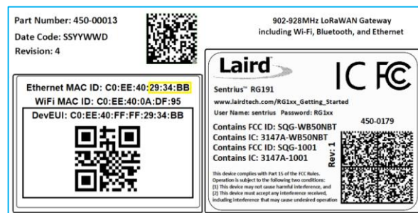
Figure 4: Bottom label (Standard GW – Left, AS923 & AU915 Region Supported/Latest Version – Right)– last three bytes of the Ethernet MAC address highlighted
