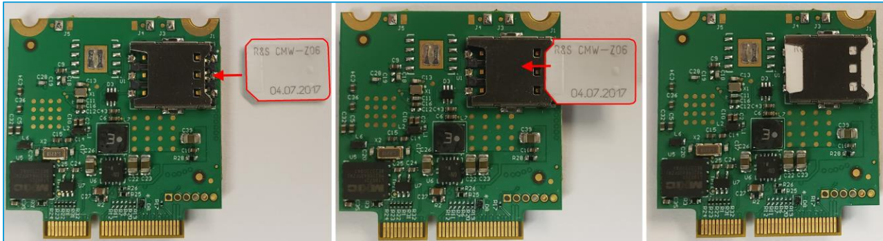
Figure 4: Insertion of nano SIM into a Pinnacle™ 100 modem (image of 453-00010)
