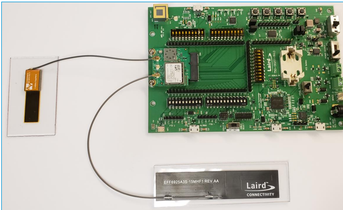
Figure 8: External antenna attachment for 453-00011 Pinnacle™ 100 modem
