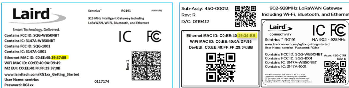
Figure 4: Bottom label (Standard GW – Left, AS923 & AU915 Region Supported/Latest Version – Right)– last three bytes of the Ethernet MAC address highlighted
