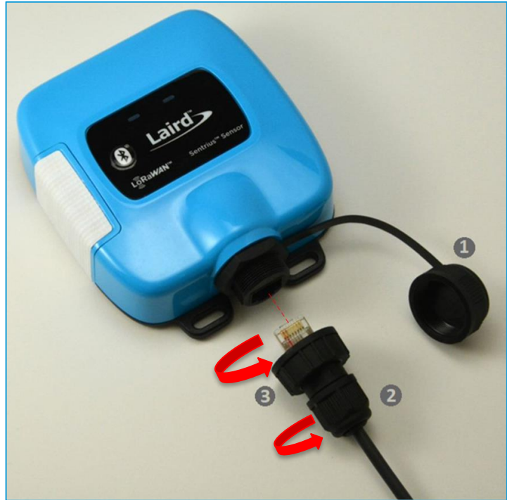
Figure 2: Installing the external temperature sensor
