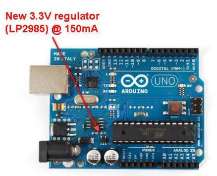
One sad thing about older boards is that they had a 3.3v power supply but it was really just whatever the FTDI chip's internal 3.3v regulator could give. You -could- get 50mA out of it, maybe. But high power stuff like XBees, SD cards, some fast ADC or DACs could easily drag down the FTDI chip and reset the USB connection. The Uno solves this problem by adding a new 3.3V regulator the LP2985 which can easily provide 150mA.
