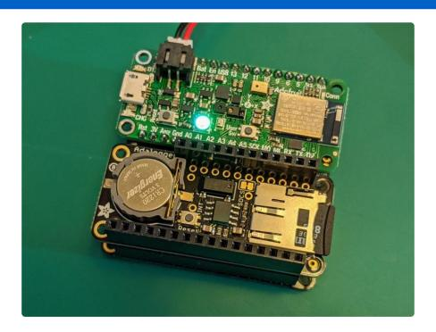
With all its built-in sensors and battery power, the Feather M4 Sense is great for datalogging projects. Stacking headers or FeatherWing Doublers need a little soldering but no custom wiring.
