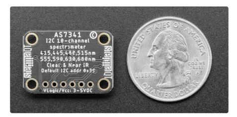
All of this capability is made accessible by mounting the sensor on a Stemma QT form factor breakout board, complete with level shifting circuitry and <a href="SparkFun Qwiic">SparkFun Qwiic</a> (https://adafru.it/Fpw) compatible <a href="Stemma QT">Stemma QT</a> (https://adafru.it/Ft4) connectors. This means that you can, without needing to solder, connect our AS7341 breakout into your 3.3V
