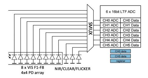
11 readable individual sensor elements (10 light channels plus flicker detection) don't exactly fit through a 6-channel ADC all at once, so the chip includes a so-called Super MUX (SMUX) that allows you to route the signal from any sensor to any ADC channel. Now that's some super multiplexing! The sensor also has GPIO and interrupt pins that can allow it to communicate directly with other sensors, or the microcontroller itself.
