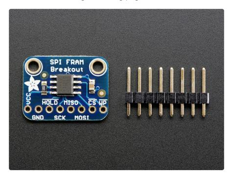
This particular FRAM chip has 64 Kbits (8 KBytes) of storage, interfaces using SPI, and can run at up to 20MHz SPI rates. Each byte can be read and written instantaneously (like SRAM) but will keep the memory for 95 years at room temperature. Each byte
