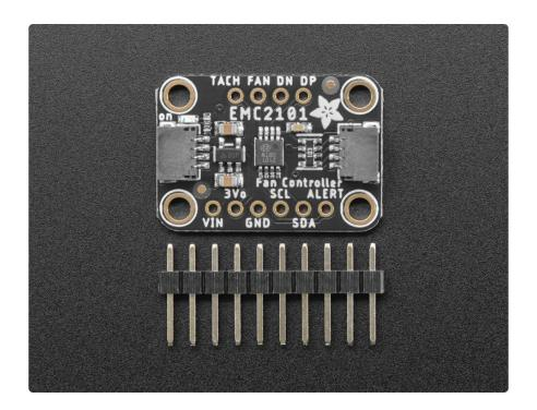
Four pin PC fans have a power and ground pin (those are often red and black) and then two more pins. One of those extra pins, the PWM pin, allows you to set a the speed of the fan. The last TACH pin is for a tachometer output that allows the EMC2101 to monitor the speed of the fan to make sure it's working as expected. Instead of using an PWM output and counter input on your microcontroller, this chip will take care of that all for you, all over every-day I2C.
