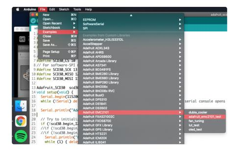
After opening the demo file, upload to your Arduino wired up to the EMC2101. Once you upload the code, you will see the Internal and External Temperature, Fan speed and PWM duty cycle values being printed when you open the Serial Monitor (Tools->Serial Monitor) at 115200 baud, similar to this:
