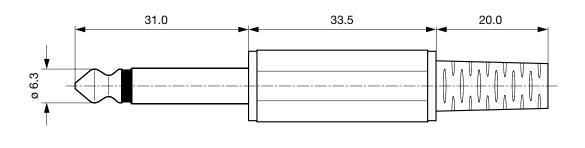
Cable diameter max. 6.8 mm
