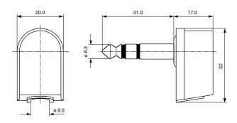
Cable diameter max. 8.0 mm
