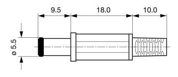
Cable diameter max. 4.0 mm
