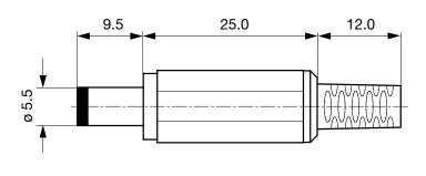
Cable diameter max. 4.0 mm
