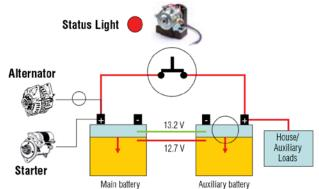
**3** When batteries reach 12.7V, the Smart Battery Isolator senses it, opens the solenoid relay to separate the battery banks, and turns off the status light. This protects the starting battery while allowing the auxiliary battery to continue to power the auxiliary loads.
