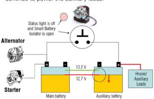
4 When the vehicle is restarted, the starting battery has enough power to crank the engine, but the auxiliary battery is significantly depleted. The Smart Battery Isolator is open and the battery banks are separated.
