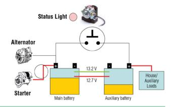
5 The engine is powering the alternator, and the starting battery has reached 13.2V. Only now does the Smart Battery Isolator reconnect, enabling the depleted auxiliary battery to be charged. By not reconnecting until the main battery is charged, the alternator is protected from excessive loads.
