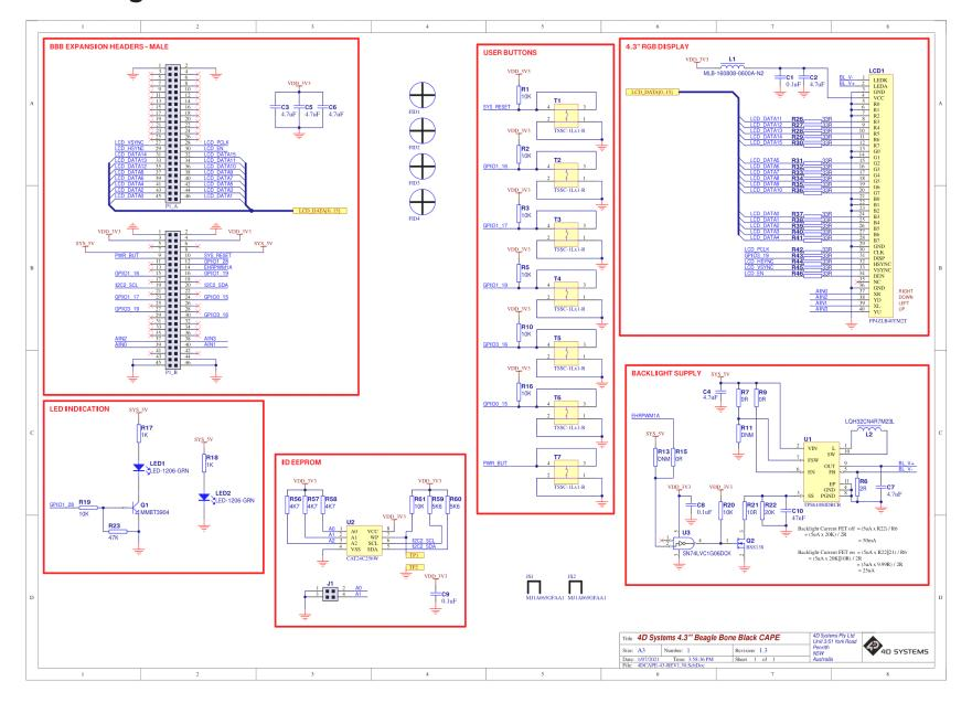
4DCAPE-43 Series Schematic Diagram 1.4
