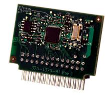
The CPM 5000 decreases product time-to-market for LonWorks® based devices. It includes all the components needed to implement a control node using the FT 5000 Smart Transceiver — the smallest, fastest, highest performance, lowest cost twisted pair LONWORKS transceiver on the market.
