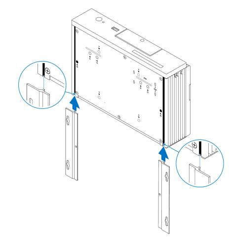
2. Secure the two mounting brackets to the back of the Embedded Box PC by using two M3x5 screws.
