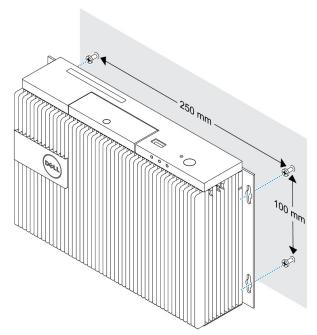
5. Secure the Embedded Box PC to the wall.
