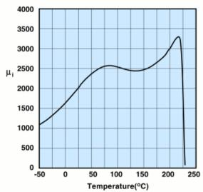
Measured on an 18/10/6mm toroid at 100kHz.
