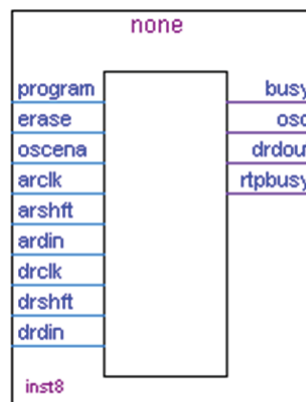
Figure 7-36. ALTUFM_NONE Megafunction Symbol for None Instantiation
