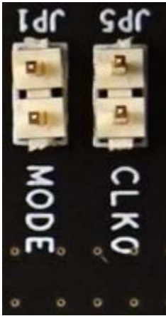
Figure 7. JP1 Jumper and JP5 Pins
