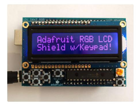
With this in mind, we wanted to make it easier for people to get these LCD into their projects so we devised a shield that lets you control a 16x2 Character LCD, up to 3 backlight pins AND 5 keypad pins using only the two I2C pins on the Arduino! The best part is you don't really lose those two pins either, since you can stick i2c-based sensors, RTCs, etc and have them share the I2C bus. This is a super slick way to add a display without all the wiring hassle.
