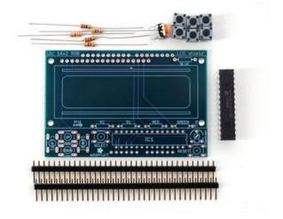
Check the kit against the parts list () to verify you have all the parts necessary
