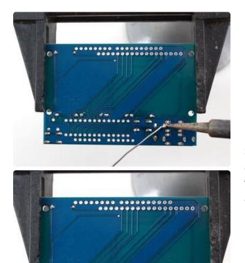
Solder each leg, taking care not to accidentally 'short' two button legs together. The ones for the directional pads are very close!
