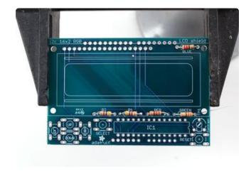
Next you can do the two 220 ohm resistors RED and BLUE - named because they are the backlight series resistors for the RGB backlights on the LCDs. These resistors are colored Red Red Brown Gold. They look very similar to the 330 ohm resistor so check carefully that you have the red-band ones. Use a multimeter if you can to verify the resistance!
