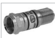
'F' Mini-Attenuator Pads Nickel Plated, Accuracy within 5%, Return Loss 20db, 22 AWG Center Pin, DC to 1 GHz Bandwidth, (M) to (F)
