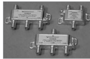
CATV Digital Ready Splitters Horizontal, 5 MHz to 1 GHz Features solder sealed back plate providing 130db RF shielding, a printed circuit design that ensures performance up to 1 GHz, and a specially plated Zinc housing and 360° port sealing sleeves allow for excellent corrosion resistance. Port spacing allows for easy installation of security shields, and each comes complete with a
