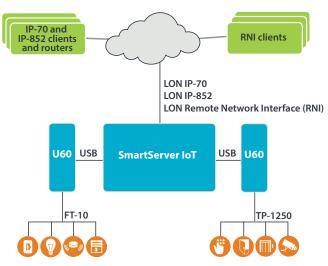
Use separate USB interface module for each channel
