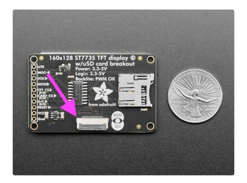
The EYESPI cables are 18 pin 0.5mm pitch flex cables. They are ~9.6mm wide, and designed to fit perfectly into the EYESPI connector. Adafruit currently offers EYESPI cables in three different lengths: 50mm (http://adafru.it/5462), 100mm (http://adafru.it/5239), and 200mm (http://adafru.it/5240).
