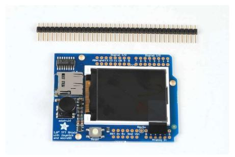
The shield comes with all surface mount parts pre-soldered. All that remains is to install the headers!
