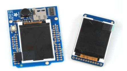
The 1.8" display has 128x160 color pixels. Unlike the low cost "Nokia 6110" and similar LCD displays, which are CSTN type and thus have poor color and slow refresh, this display is a true TFT! The TFT driver (ST7735R) can display full 18-bit color (262,144 shades!). And the LCD will always come with the same driver chip so there's no worries that your code will not work from one to the other.
