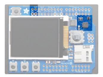
Instead of taking up a bunch of GPIO pins to read the buttons and joystick, as well as controlling the TFT backlight, we use an I2C expander chip called the **seesaw**. It is connected to the SDA/SCL pins and can read/write pins with our library. This saves a ton of pins and then you can always use the I2C pins for other sensors, as long as the address doesnt conflict
