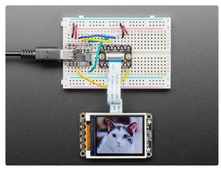
This display now comes with an **EYESPI connector**. This connector allows you to connect your display without soldering. There are <u>EYESPI cables</u> (https://adafru.it/ 18eT) available in multiple lengths, which means you can find one to fit any project. This is especially useful if your project requires the display to be freestanding, and not tied directly into a breadboard. Inspired by the popularity of STEMMA QT, it provides plug-n-play for displays!
