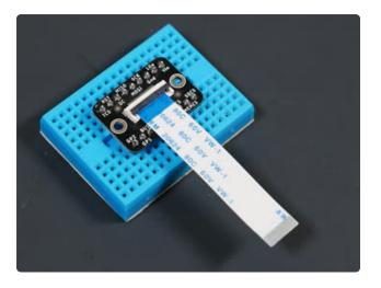
To secure the cable, lower the FPC connector latch onto the EYESPI cable.
