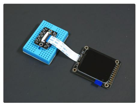
You can connect an EYESPI compatible display to the EYESPI breakout board using an EYESPI cable. An EYESPI cable is an 18 pin flexible PCB (FPC). The FPC can only be connected properly in one orientation, so be sure to follow the steps below to ensure that your display and breakout are plugged in properly.
