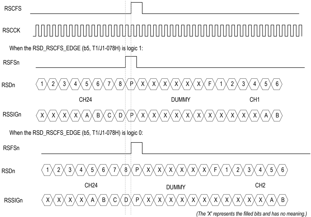
Figure 30. T1/J1 Receive Clock Slave External Signaling Mode - Functional Timing Example 3
