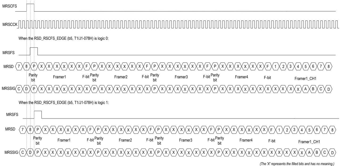
Figure 34. T1/J1 Receive Multiplexed Mode - Functional Timing Example 2
