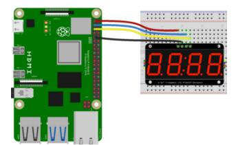
Raspberry Pi 3.3V to 7-Segment Display VIN (red wire) Raspberry Pi GND to 7-Segment Display GND (black wire) Raspberry Pi SCL to 7-Segment Display SCL (yellow wire) Raspberry Pi SDA to 7-Segment Display SDA (blue wire)
