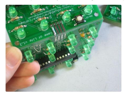
Bend the wire down and solder it to the second board.
