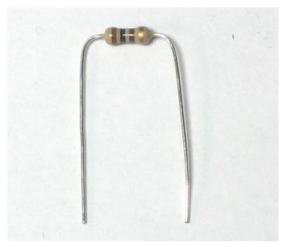
The first step is to solder in the resistors. The resistor is the tan-with-stripes things, they're probably on tape as that's how they come from the factory. Remove the tape and bend the resistors into staples as shown.
