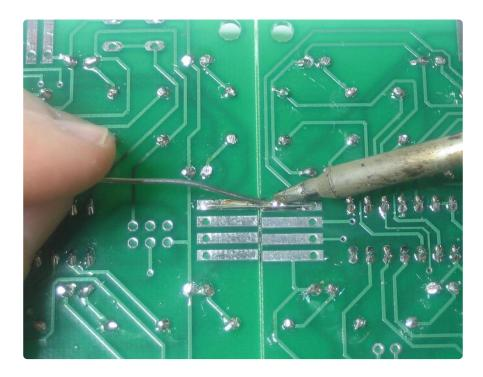
Then turn over and solder the other side too. This is a permanent connection, so make sure to use lots of solder on both sides to get a nice strong connection.
