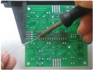
The socket has short legs so it's more likely to slip than a resistor. The easiest way to solder the socket is to hold it against the PCB with one finger (or tape) then solder in two points on opposite sides. Once you've got it tacked, solder in the remaining pins.
