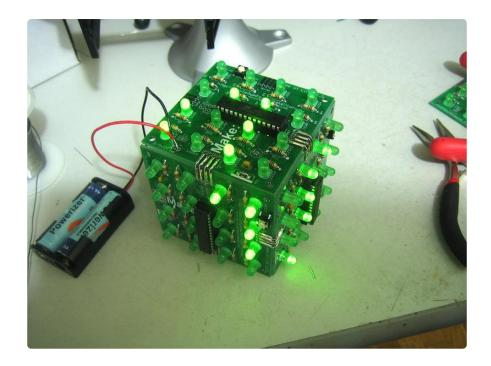
When you're done you can attach the battery pack pack and stick it onto the inside.
