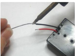
You'll have to tin the ends if you clipped the wires. Heat up the wire and dab some solder, which should wick into the wire and keep the strands from flying out.
