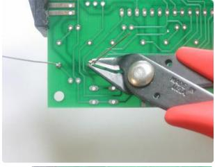
Put down the iron and pick up the diagonal cutters. Using the cutters, clip the wires of the resistor right above the joint.
