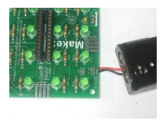
Next, connect up the battery pack. The red wire of the pack goes to the hole marked with a +, the black wire goes to ground, marked with a -.
