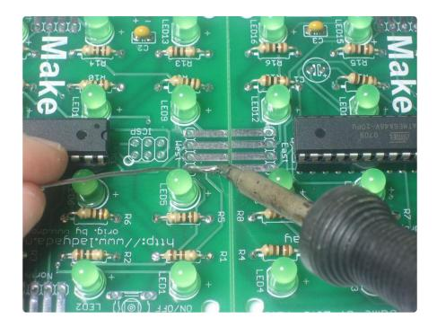
Then drag the soldering iron between the two boards, and slowly lift it in the middle.
