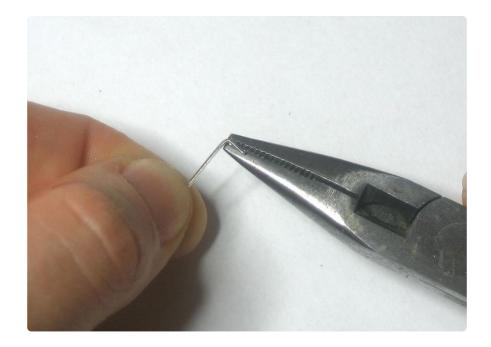
Thread it through the adjacent holes, then solder to make a connection to both boards.
