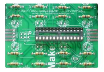
The socket has a little note in one end, make sure this matches with the little notch in the silkscreened PCB image. In the picture shown, the notch is on the left.
