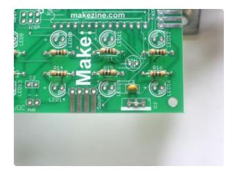
Next we're going to place the ceramic capacitor C3 and the wire jumper for IC2.
