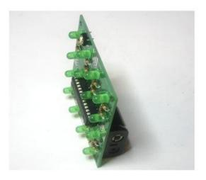
Stick the battery pack onto the back of the PCB, near the bottom. That way the weight of the batteries will act as a stand so that the kit can sit on your desk!
