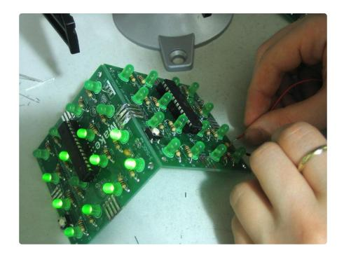
Connect a third board. The trick to knowing how to orient boards is that you can always connect North and East & South and West ports together. In this case we connect West and North of the new board to the existing structure.
