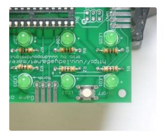
Place the ON/OFF/Reset button. The button is non-polar. The button will snap in and should sit flat against the PCB.
