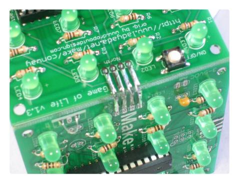
Test the two boards by touching the battery case to the + and - on one of the boards. The game should play on both boards.
