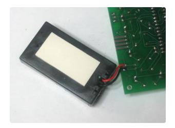
Time to wrap it up. Remove one side of paper from the sticky foam, place it in the center of the battery holder. Then remove the other side.
