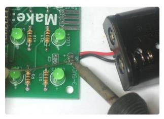
Solder in the two wires.
