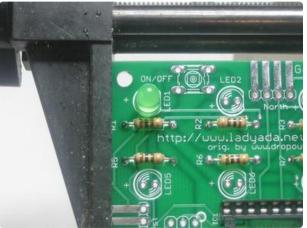
Next are the LEDs. LEDs, unlike resistors, are polarized and must be placed correctly or they won't light up. One leg of the LED is slightly longer than the other. This is the positive (+) leg. If you look at the image on the PCB, you'll note that one side has a + next to it, this tells you how to orient the LED. Make sure the long lead goes in the hole marked +.
