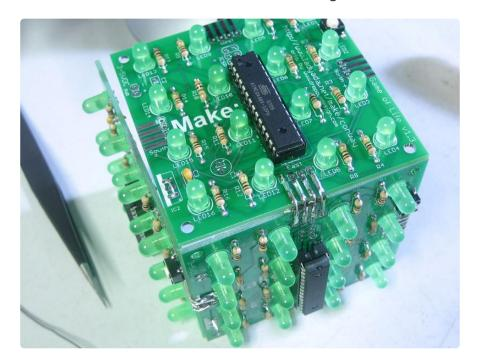
Test the cube after each new board to make sure you've got it on right.
