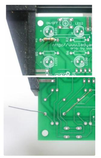
The resistors are named R1 thru R16. Placing them on the PCB is easy, just look for the image on the PCB that matches the shape of the resistor. Resistors are non-polarized that means you can stick them in 'either way' and they'll work just fine.
