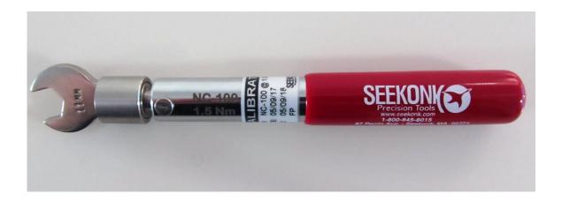
Pre-set at factory to desired value within a +/- 4% tolerance. When preset torque value is achieved, a distinct click is felt and heard, followed by a sudden release into several degrees of free movement. Ideal for applications in which one torque value is used extensively. Compact design makes these tools invaluable in hard to reach locations. Tools automatically reset when torquing- force is removed.
