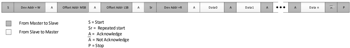
Figure 22. Master I 2 C Initialization Mode
