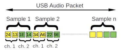
The length of a complete audio packet is equal to the bits per sample rounded up to bytes, multiplied by the number of channels and the sample rate, then divided by 1000 as a packet is sent every millisecond. For a sample rate of 48000, 16 bits per sample, 2 channels the calculation is as follows:
