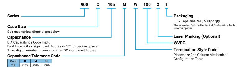
The above part number refers to a 900 C Series (case size C) 1.0 MFd capacitor, M tolerance (±20%), 100 WVDC, with W termination (Tin/Lead, Solder Plated over Nickel Barrier), laser marking and ATC Matrix Tray packaging.
