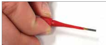
Plastic tool with contact in proper position.
