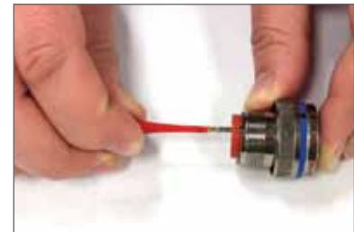
Plastic tool with contact in proper position.
