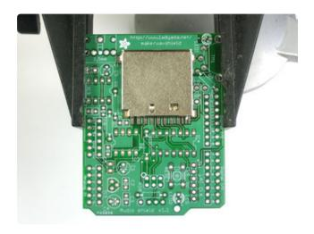
We're going to the SD card first. While surface mount parts are a little tougher than thru-hole, this piece has pin spacing of 0.1" so it is quite easy. Doing it first also gives us lots of working room.
