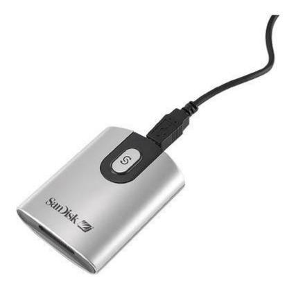
These are very common, available in any computer store. The shield **doesn't** have the ability to display the SD card as a 'hard disk' like some MP3 players or games, the Arduino does not have the hardware for that, so you will need an external reader!
