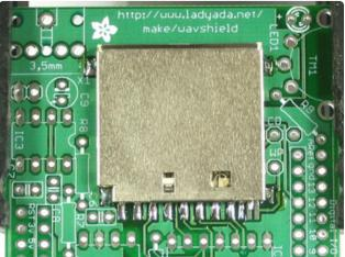
Now go thru and solder the 8 leftmost pins that stick out from the holder. The three rightmost pins are thinner and closer together so they are tougher to solder. Luckily they are not used and you simply skip them (although the photo shows them done).
