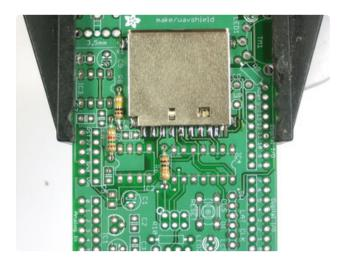
Finish up the resistors by placing **R8** (100Kohm), and **R7** (1.5K)
