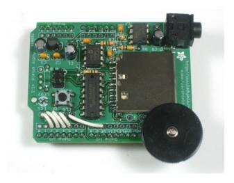
Pins 13, 12 and 11 are used to talk to the SD card and cant be changed. The rest of the pins, however, are more flexible. Still, for all the examples on the site we'll be using this wiring, so it is suggested to just go with this.
