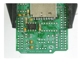
Next is the DAC (digital-analog converter) IC2. This is what turns the data into music. Make sure you pick the DAC to solder in here, it says MCP4921 on it and has a stylized M.
