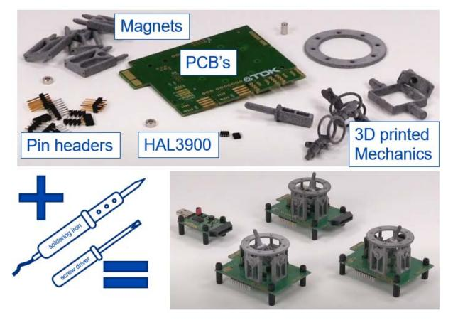
The TDK JOYSTICK Eval. Base Kit V1.0 is intended to connect TDK Hall Sensor HAL 3900 in a Joystick like setup to programming hardware, there are three options.
