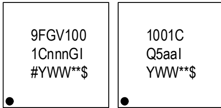
Figure 9. 9FGV1001C Marking Diagrams
