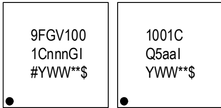
Figure 9. 9FGV1001C Marking Diagrams
