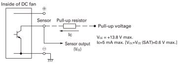
Output waveform (Need pull-up resistor)
