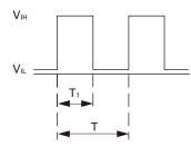
$\begin{array}{l} V_{IH}=4.75 \ to \ 5.25 \ V \ \ V_{IL}=0 \ to \ 0.4 \ V \\ PWM \ duty \ cycle \ (\%) = \frac{T_1}{T} \times 100 \qquad PWM \ frequency \ \ 25 \ (kHz) = \end{array}$ Current source (Isource) = 1 mA max. (when control voltage is 0 V) Current sink (Isink) = 1 mA max. (when control voltage is 5.25 V) Control terminal voltage = 5.25 V max. (when control terminal is open) When the control terminal is open,
