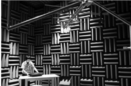
Acoustic radio wave anechoic chamber
