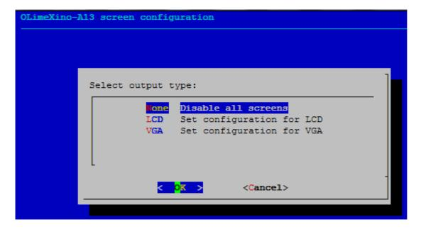
Choose the resolution and the interface (LCD or VGA). Note that VGA output is hard to implement and requires both additional hardware and good soldering experience.
