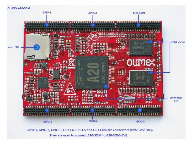
Please note that there might be differences in the layout of top of the board compared to the latest revision. One of the notable changes introduced in hardware revision C of the design, is the addition of GPIO-6 row of pinholes that provides easier access to some additional pins. The general routing and memory positions are also adjusted.
