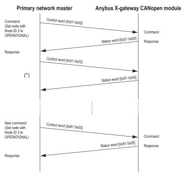
$(^\star)$  The communication is performed in an ongoing ping-pong fashion. The same command is sent repeatedly, but as long as the toggle bit is not changed, the module will ignore the message. A new command is signalled by the toggle bit changing value.
