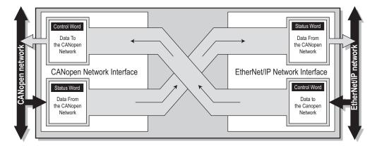
Each buffer holds up to 512 bytes of data, where the first two bytes on the primary network side always are used for control/status information. The remaining 510 bytes gives the theoretical upper limit for the number of data bytes that can be exchanged in each direction. Please note that the actual number of bytes that can be exchanged is highly application and network dependent and can thus be noticeably less than 510 bytes.
