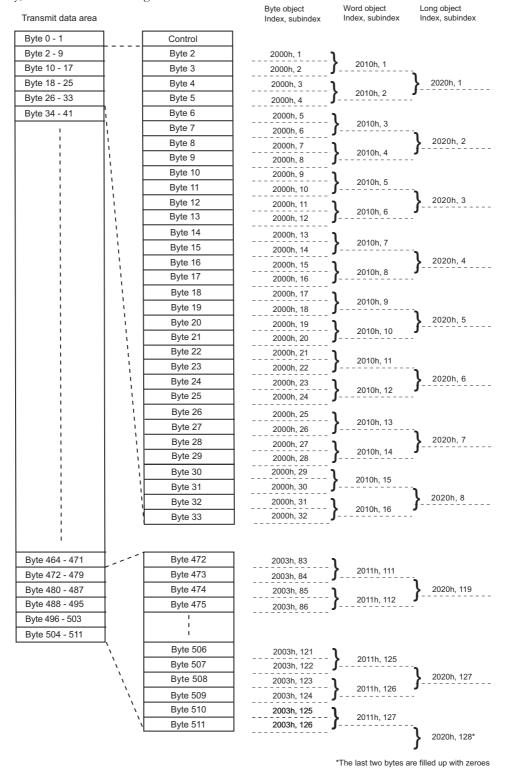
Note 1: The picture shows the Transmit data area. The Receive data area has the same structure, but with indices for byte objects starting at 2100h.
