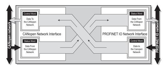
Each buffer holds up to 512 bytes of data, where the first two bytes on the primary network side always are used for control/status information. The remaining 510 bytes gives the theoretical upper limit for the number of data bytes that can be exchanged in each direction. Please note that the actual number of bytes that can be exchanged is highly application and network dependent and can thus be noticably lower than 510 bytes.
