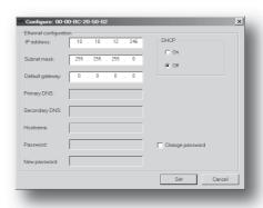
Optionally, the configuration may be protected from unauthorized access by a password. To enter a password, click on the 'Change password' checkbox, and enter the password under 'New password'. When protected, any changes in the configuration requires that the user supplies a valid password.
