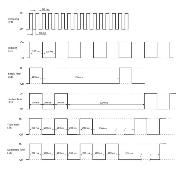
When LSS services are in progress, both the ERR LED (red) and the RUN LED (green) are flickering.
