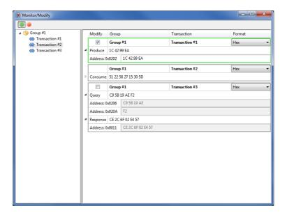
If Modify is enabled, it is possible to change the data values during runtime in Produce transactions and in the Query part of Query/Response transactions, i.e. only the out area of the Communicator can be modified. This will inhibit any data from the industrial network (CC-Link), but input data from the CAN network will still be updated.
