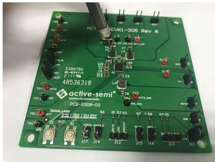
Figure 4—Measuring output voltage ripple
