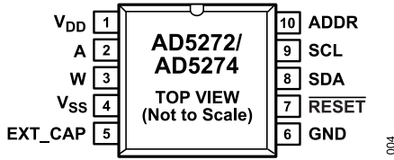
Figure 4. MSOP Pin Configuration
