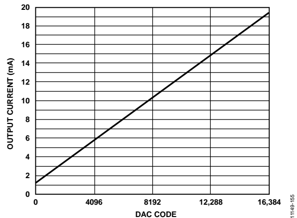
Figure 151. Gain Curve for FSC_x[9:0] = 512, DAC Offset = 1.228 mA
